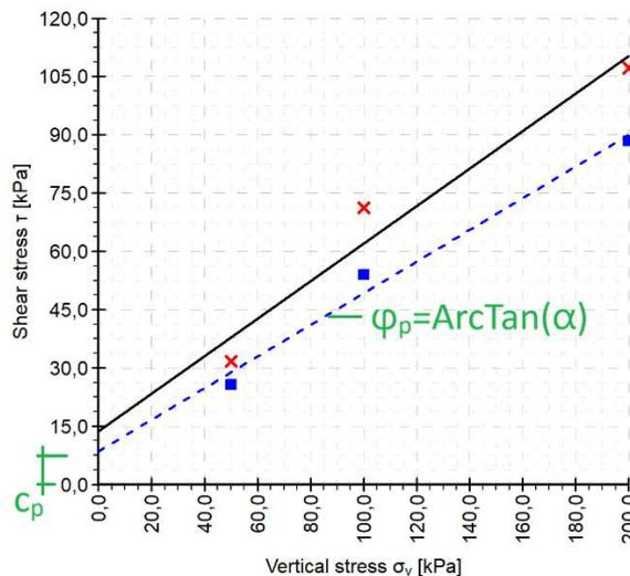
*Note: We usually look for the stated value of the shear parameters in the part of the test beyond its peak in an attempt to find residual shear strength parameters. However, since the shear box test is not suitable for determining the actual residual parameters, we present the derived shear parameters for the selected deformation.*
