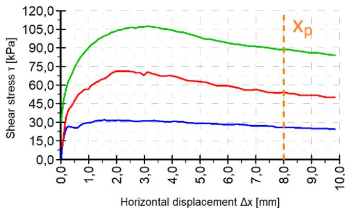
We then fit a straight line through the obtained points and calculate the values  $\varphi_p$  and  $c_p$ .
