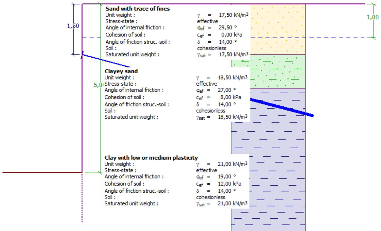
*Scheme of the anchored wall from pile sheeting – assignment*
