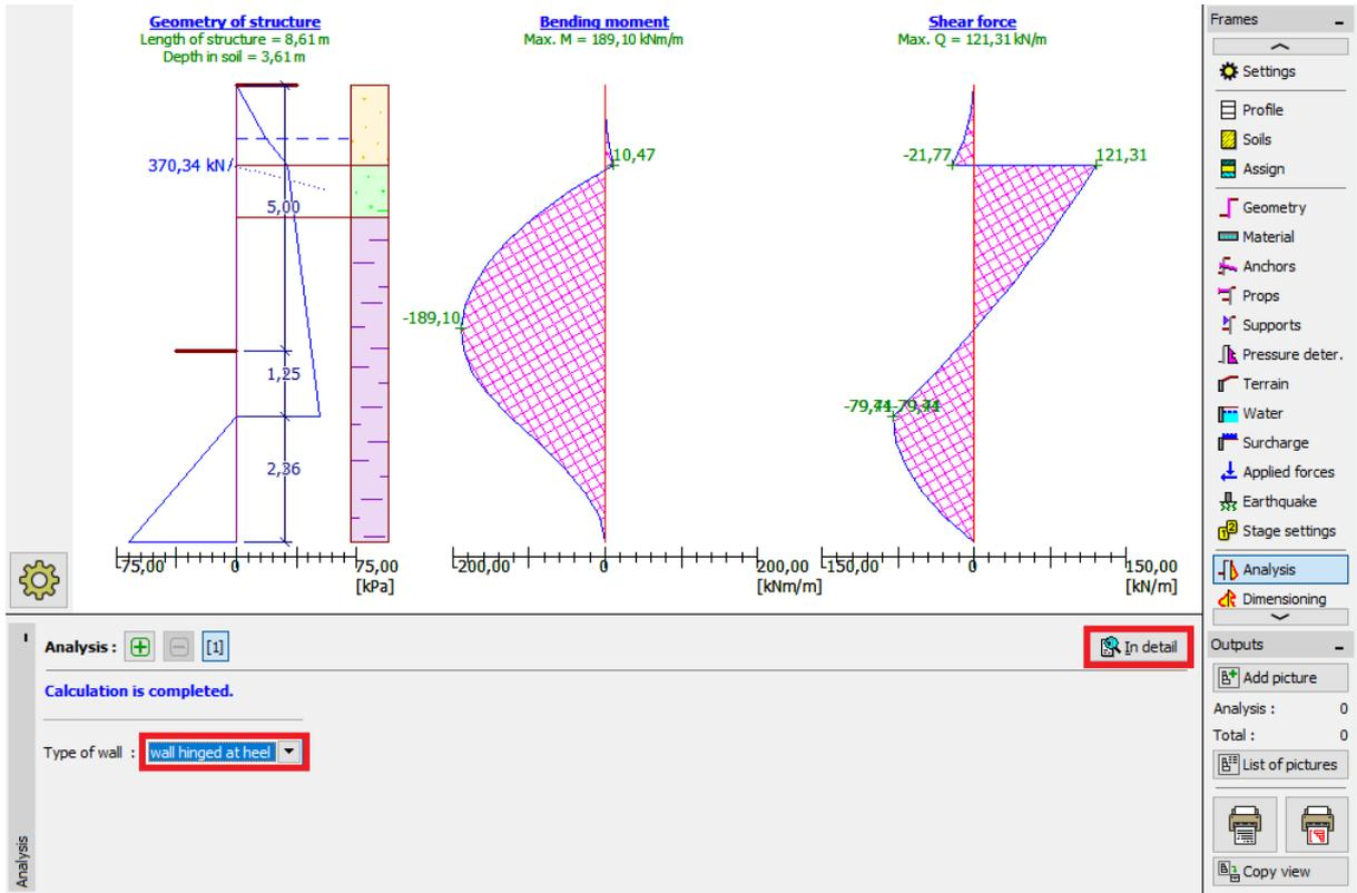
“Analysis” Frame – Construction stage 1 (Wall hinged at heel)
