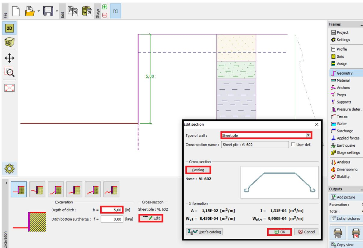
“Geometry” Frame – depth of the ditch and cross-section selection
