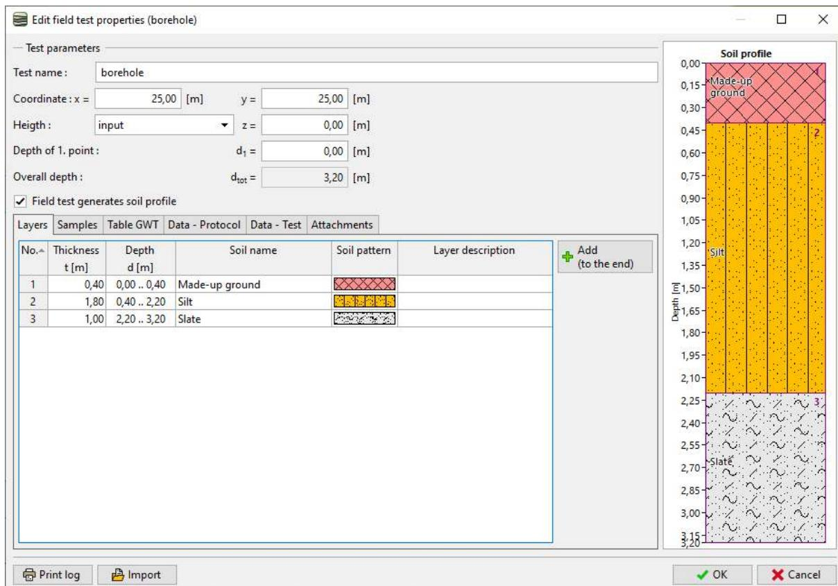
In the „Soils“ frame, we will create a list, by clicking the „Adopt from field tests“. For individual soils, we can change the bulking coefficient (important for the calculation of excavation volumes) and other soil parameters, that are needed in the calculation programs.
