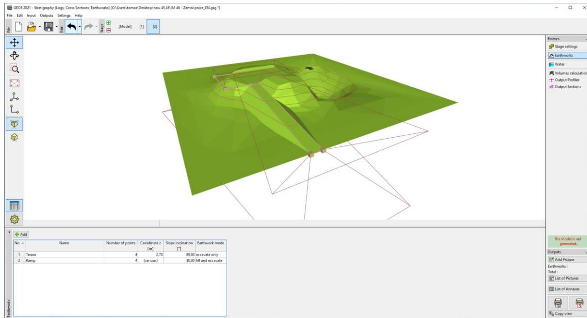
We will go to the “Water” frame and input the height of the water level in the pond ( $z = -0.4\text{m}$ ). The water level is represented only by one point anywhere in the model. The created water level is then horizontal.
