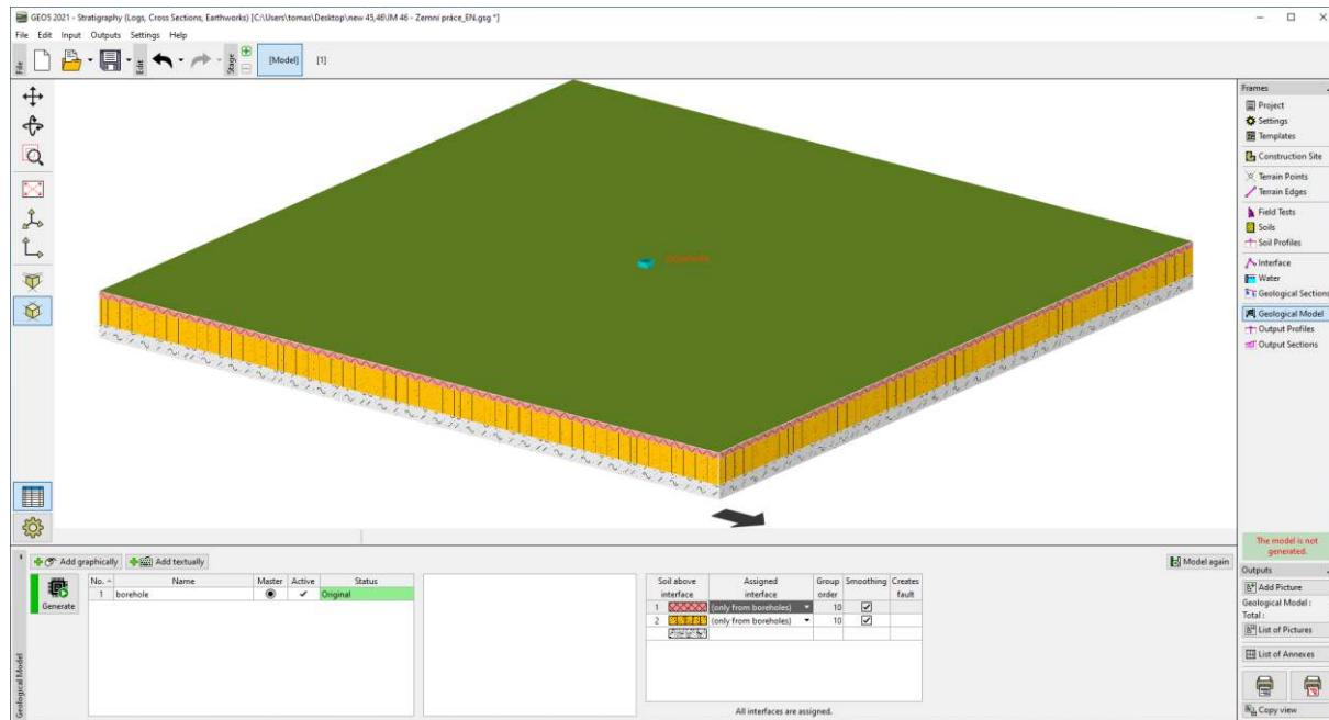
We will switch to the first construction stage. In the „Stage Settings“ frame, input the terrain modeling mode in the given stage. We will choose the „Terrain points and edges“, because we already have the points focused.
