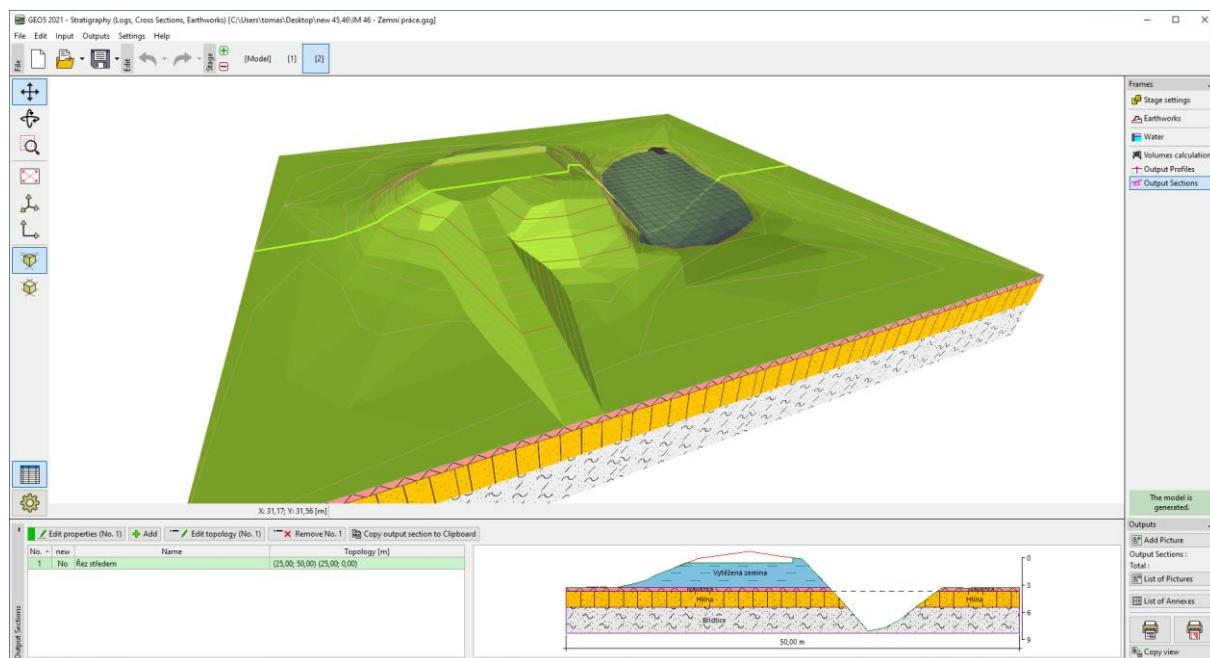
In the „Construction Site“ frame, we will enter the dimensions of the model. We assume a square shape with a length of 50 m. The minimal x and y coordinates will therefore be 0m and maximum 50m.
