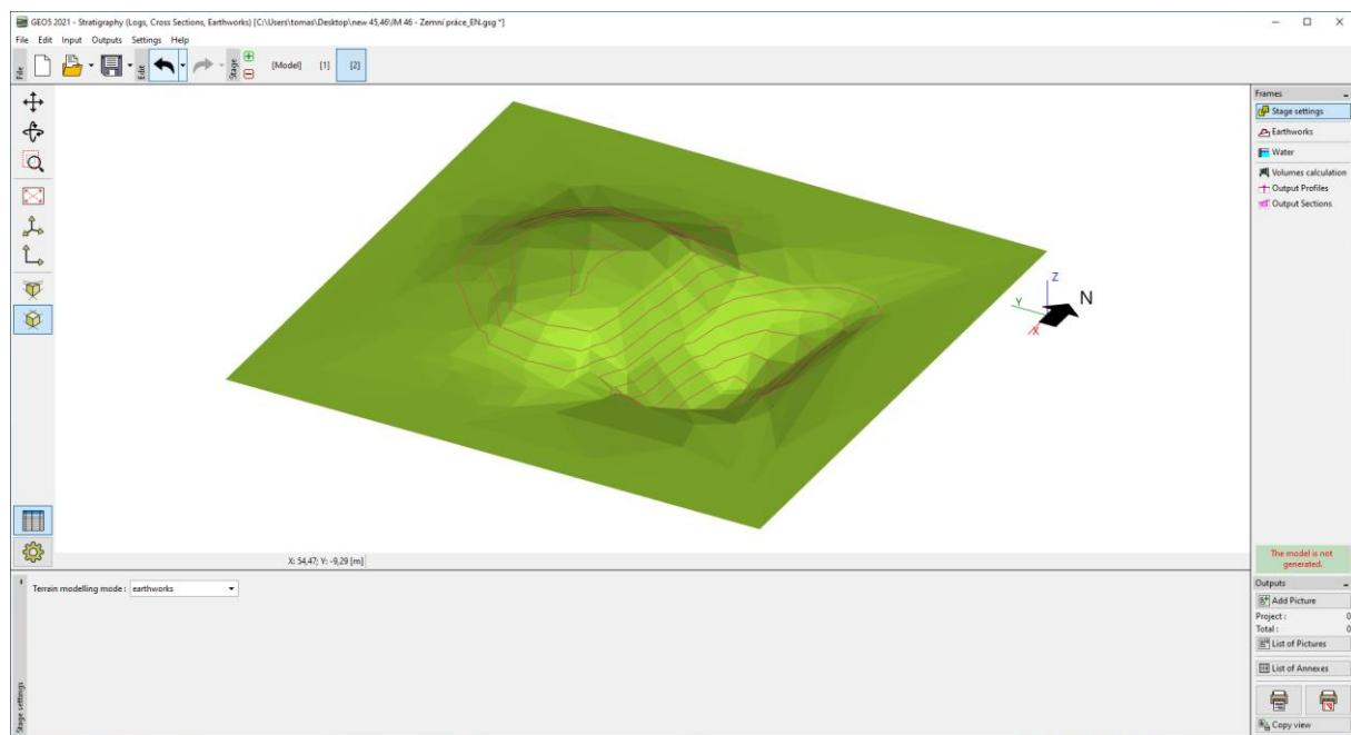
In the “Earthworks” frame, enter the shape of the terrace. In our case, we will choose rectangle, with the coordinates: [19;40], [19;25], [28;25], [28;40] and height of 2,7m. Because the edge will be vertical, we enter a slope of 89 degrees. (90 degrees cannot be enter, due to construction principles). Enter the adjustment as „only excavate“ – the adjustment will only remove the soil.
