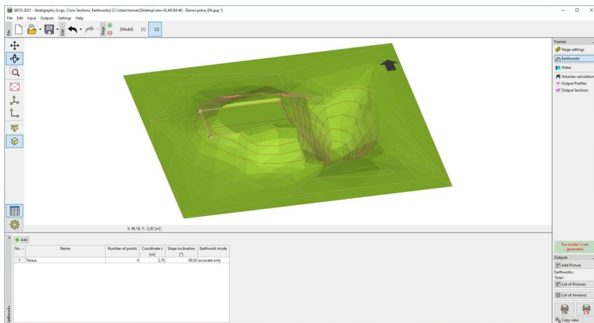
We will enter another earthwork, this time representing the access ramp. For simplicity, we will choose a rectangle with coordinates: [28;35], [50;35], [50;33], [28;33]. The height of the adjustment is a variable this time – at the top, the height is 2.7m, down it is 0.0m and a slope of 30 degrees. We will be adding and removing the soil this time – therefore, we will choose the mode: „Fill and excavate“ mode.
