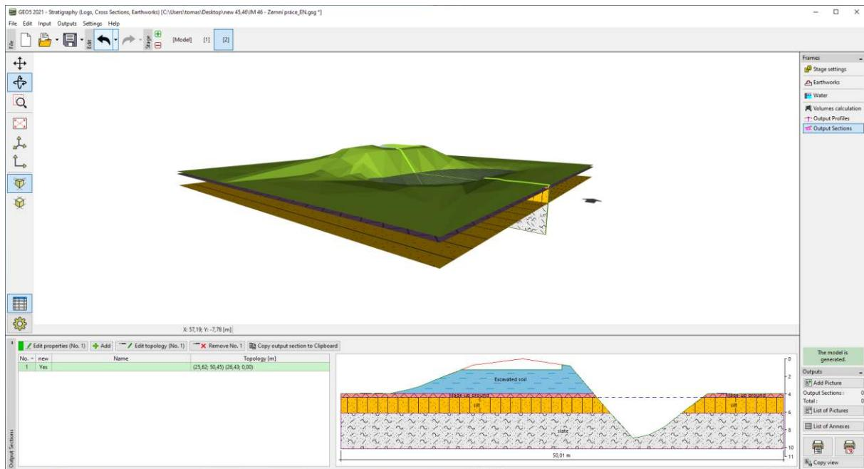
Then we will go to the “Slope Stability” program (menu item „Edit“ „Paste data“), where we will insert the cross-section. After entering the soil parameters, surcharge, and calculation parameters, we can then analyse the construction.
