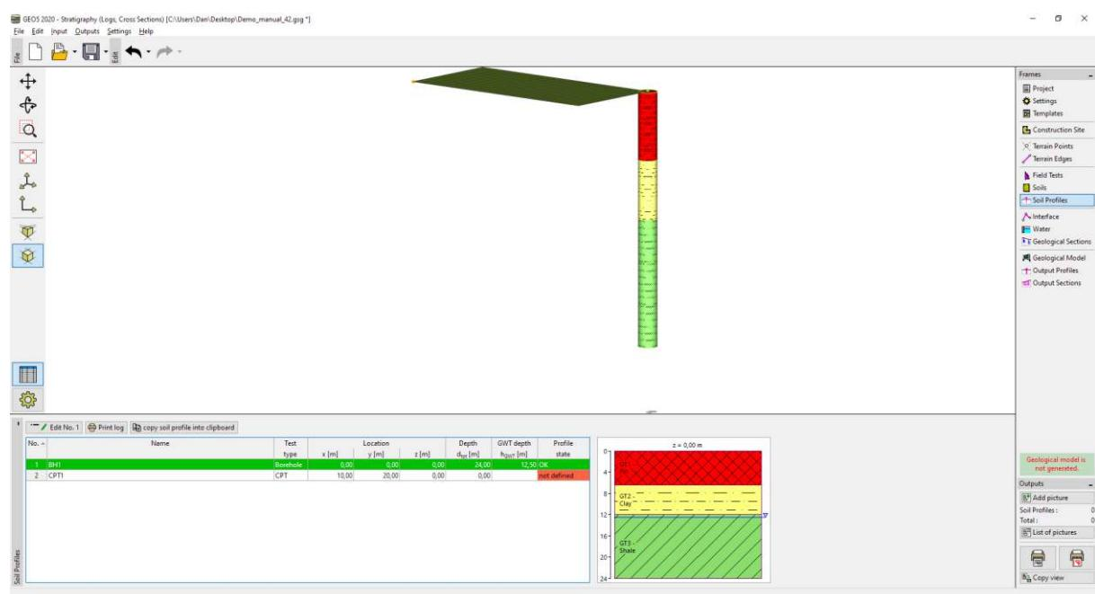
Next, we will interpret the CPT. When the dialog box opens, the program evaluates the CPT test by the Robertson method and will design the soil layers.
