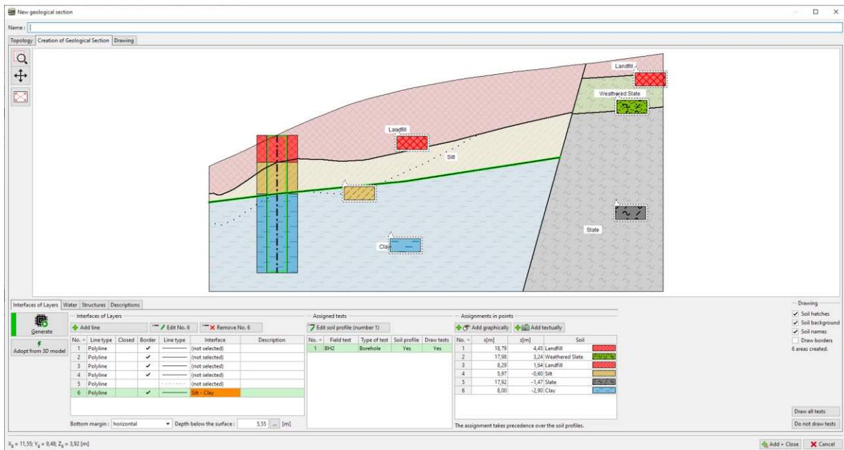
We will also adjust the landfill interface. This time, we will delete the old interface and create a new one. This procedure is simpler, but we will lose the information about the original shape. In this case, after deleting the interface, we will also need to extend the line, which creates the fault so that the areas are closed.
