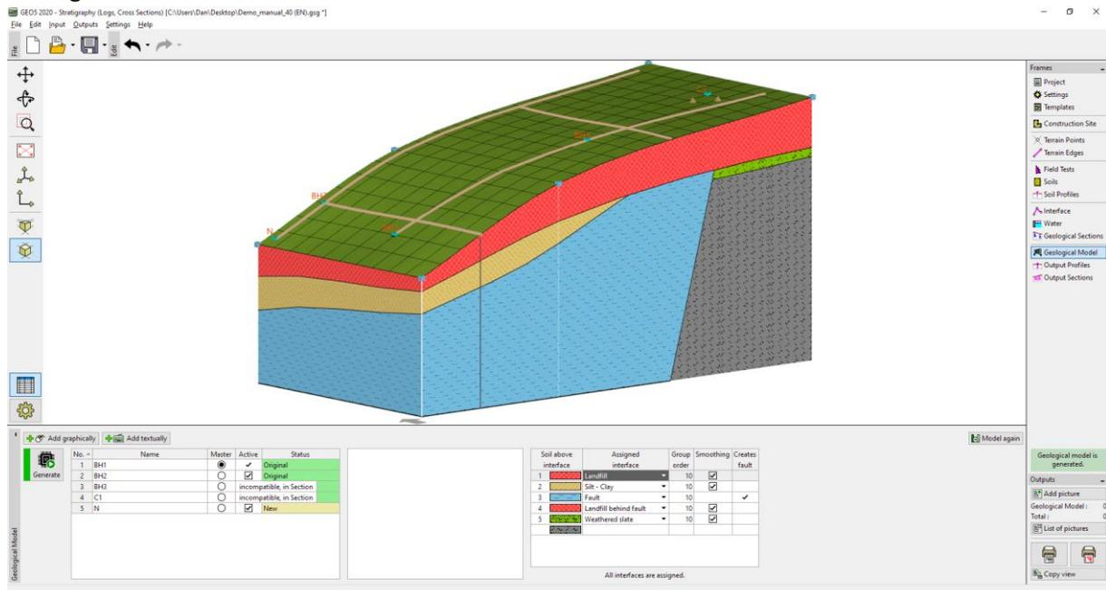
We will, therefore, adjust the order of layer generation. First, we will generate the fault, that will divide the model into two areas.
