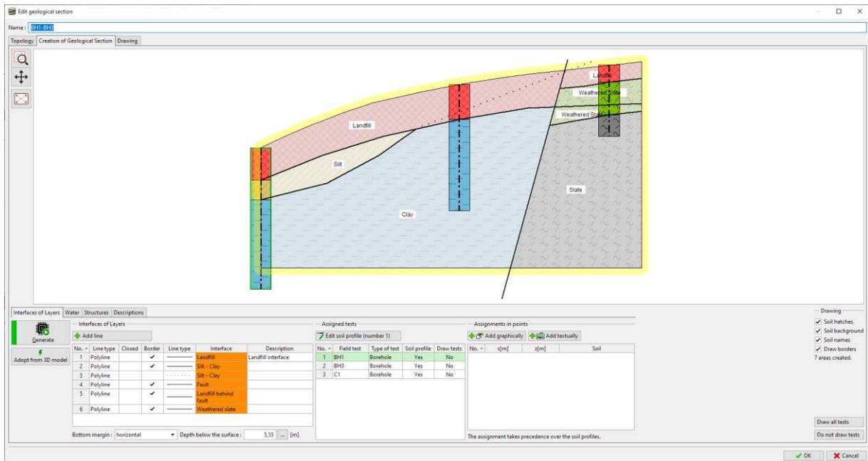
We will go the geological model frame. The number of soils, resp. interfaces between the soils remains the same as in the previous example. It is necessary to add new soils to the master borehole. The number of soils and their layers is always given by the master borehole.
