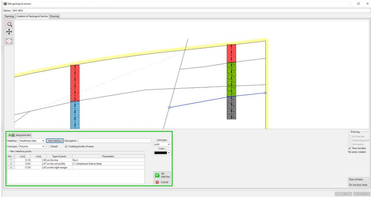
This completes the section. Although the landfill interface divides the weathered slate layer, the model generation will not be affected by it.
