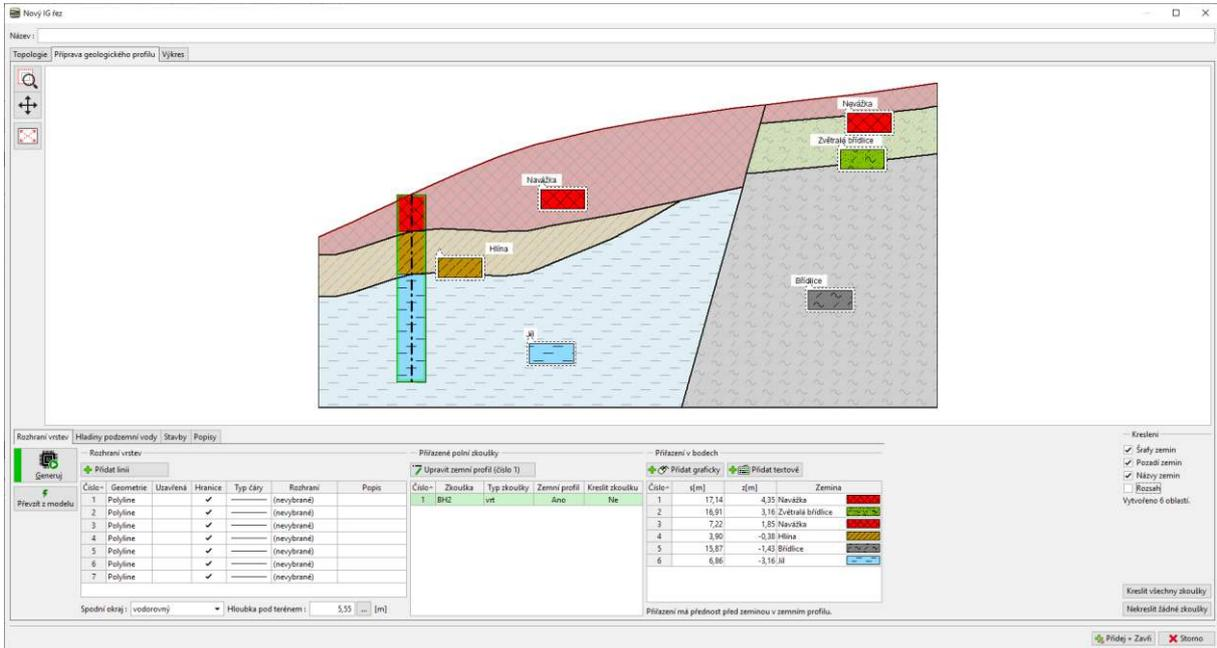
We will adjust the interface between the silt and clay. Select the line, and mark it as auxiliary (it will appear dotted) and turn off the "Creating border of areas" checkbox. We could delete this line too, but we want to see it when constructing a new one.
