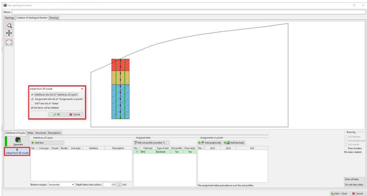
Soils are now assigned by using points in each area. Interfaces are not assigned to the individual lines so that they do not create additional points in the interfaces of the 3D model.
