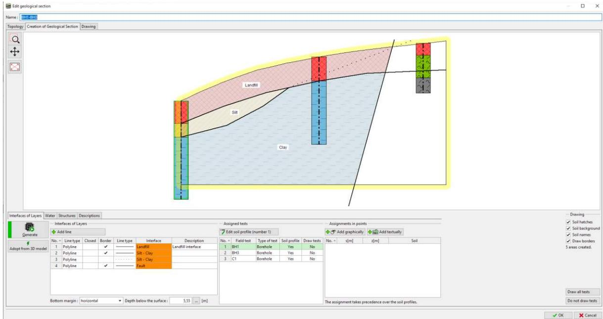
We enter the interface behind the fault and assign it a new interface (Landfill behind fault)
