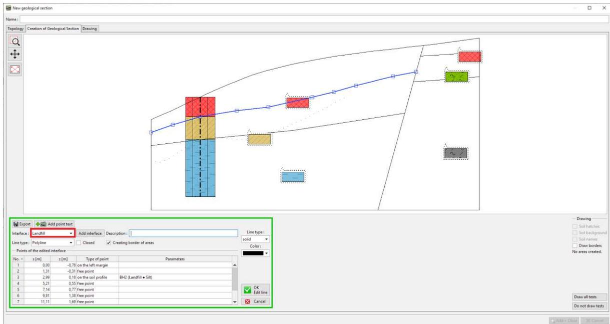
*Note; The 3D model is only affected by points that have assigned interfaces. If we want to keep the exact shape of the interface in the 3D model, we might need to model the interface by more points – even if the section is straight.*
