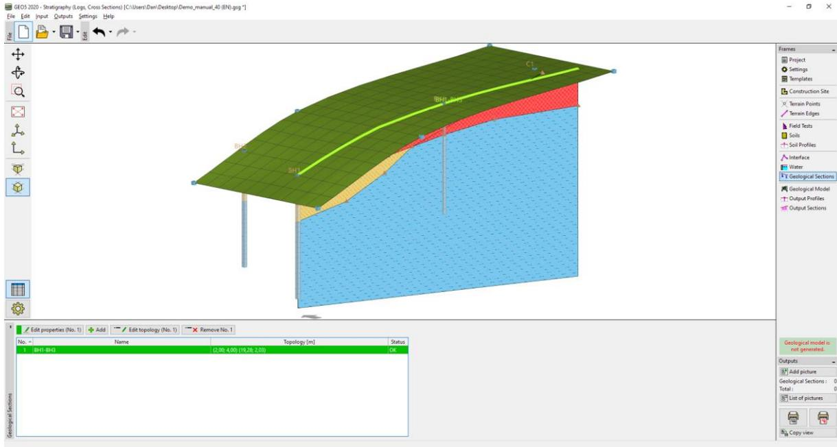
We will add the C1 borehole to the geological section.
