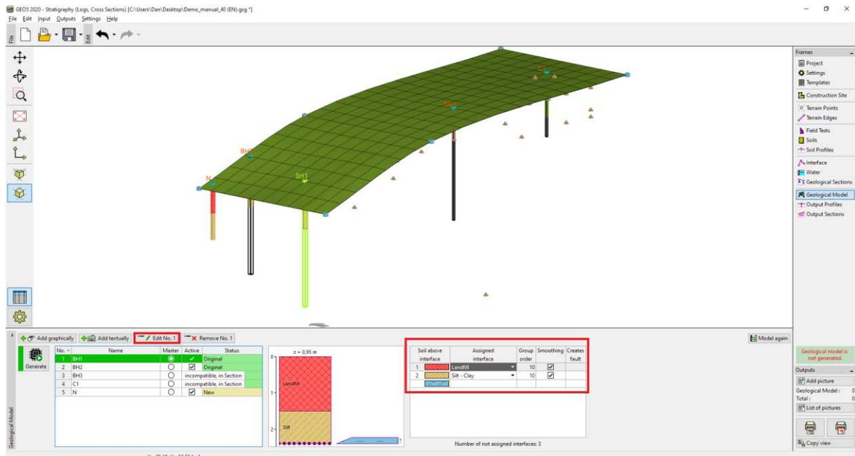
We will open the window for editing the master borehole and add new soil behind the fault (from top to bottom). As we do not know the position of the layer interface in the borehole (or there is no interface at all), we will leave the location type as “not defined”
