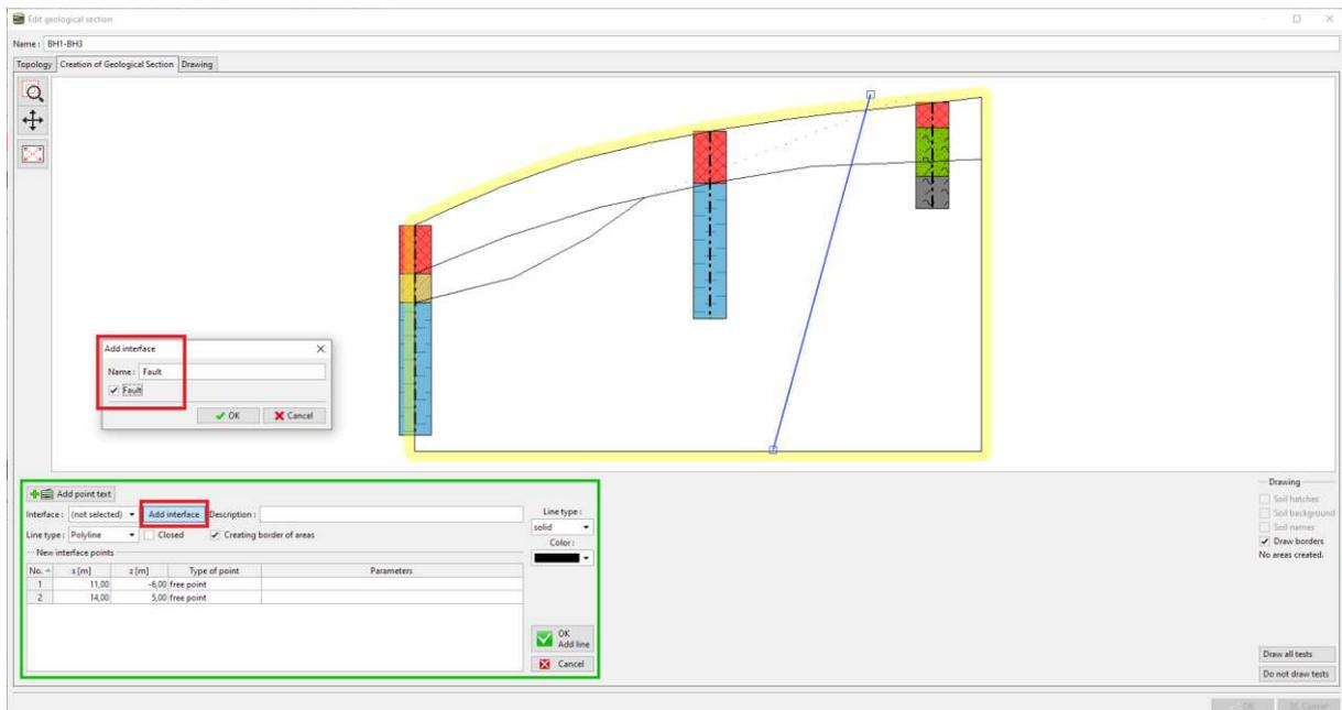
After the generation of sections, only the soils located to the left of the fault are assigned.
