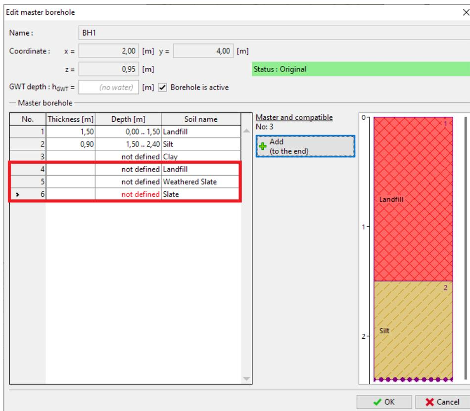
The layer table has now changed. We will assign the fault interface and other soil interfaces behind the fault.
