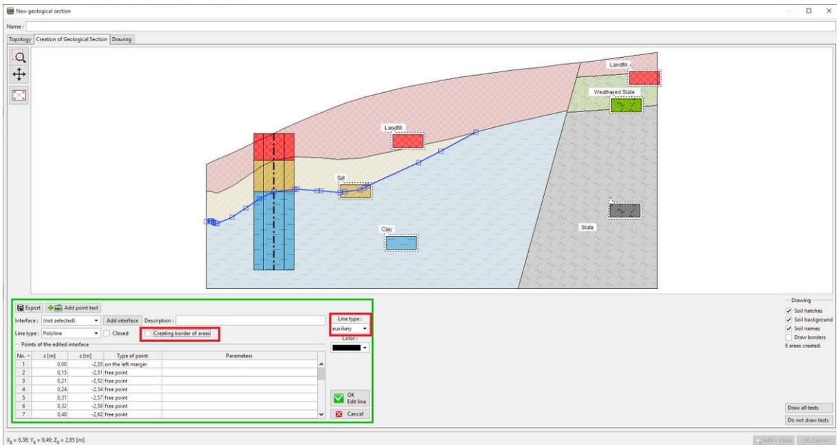
We will enter a new shape of the interface and assign it the "Silt-clay" interface
