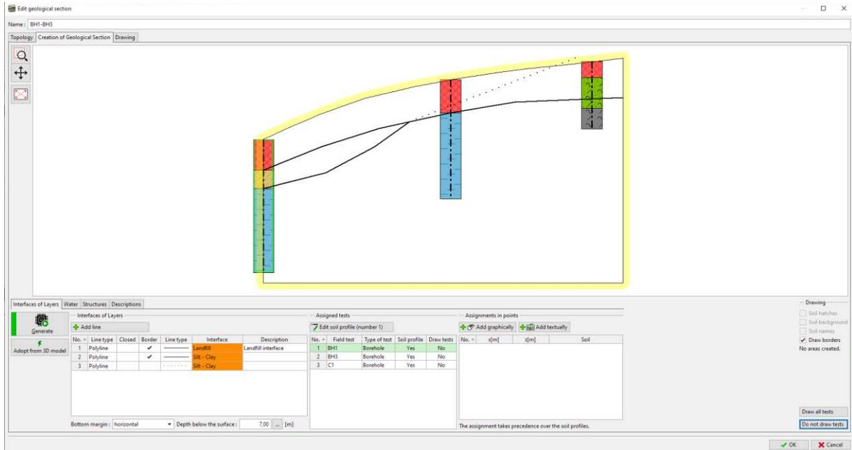
We will enter a fault – add a new interface and check the Fault checkbutton.
