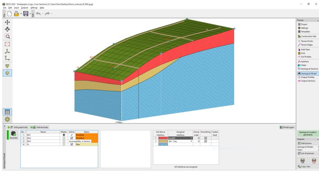
During an additional geological survey, a borehole C1 was carried out at the [18,4]. The borehole found a layer of backfill 0.8 m thick, then a 1.5 m thick layer of weathered slate, and was ended in a strong slate. The task is to adjust the model so that it respects the findings and also fully corresponds to our ideas of geology in the area.
